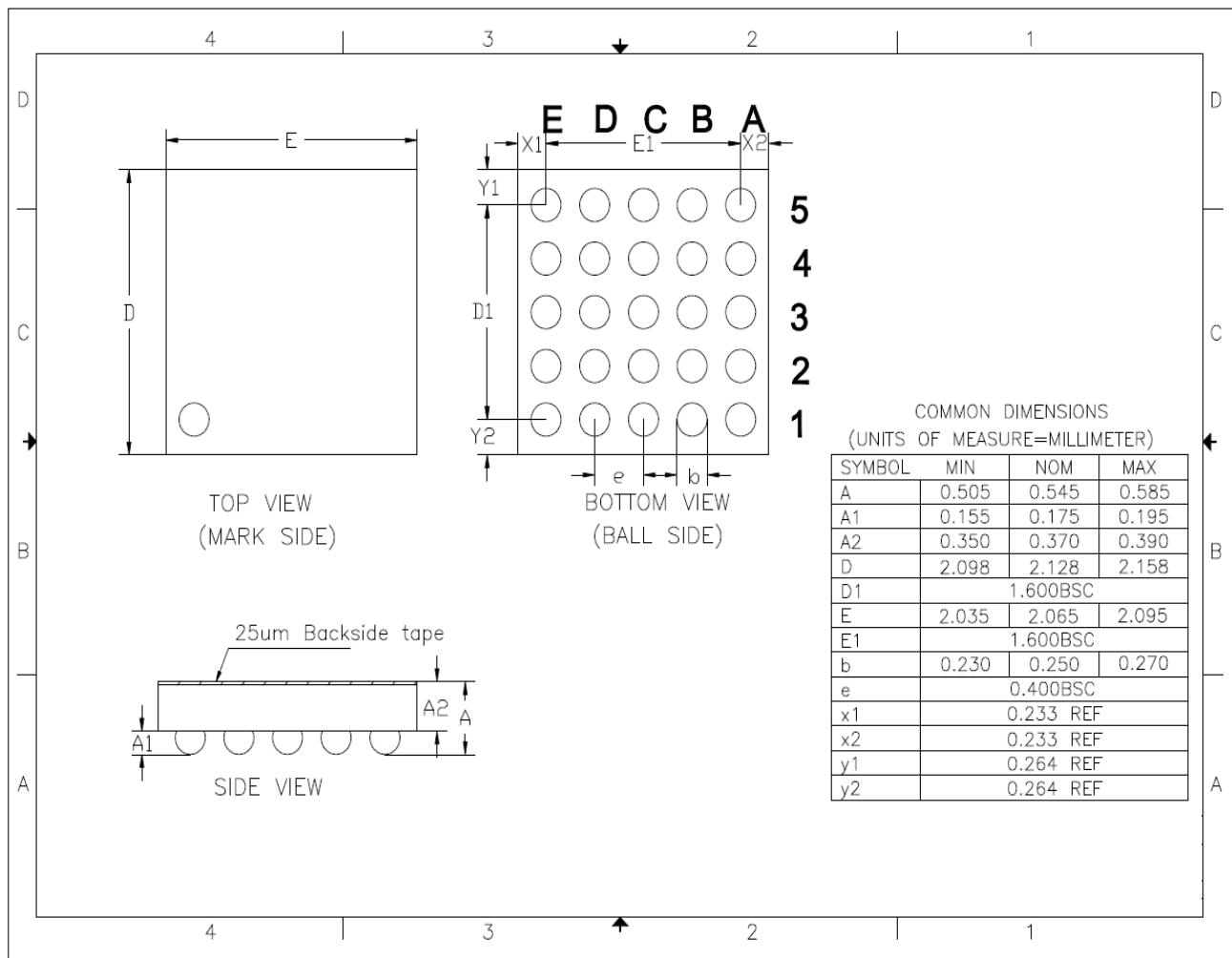
Figure 5-10 WLCSP25 Recommended footprint <sup>(1)</sup>
