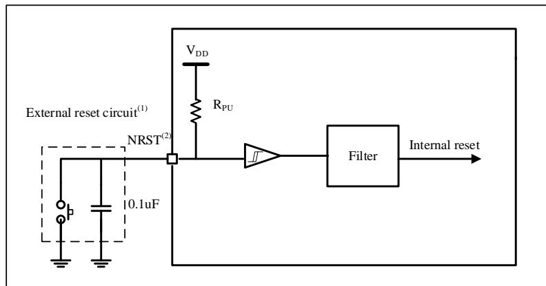
1. The reset network is to prevent parasitic reset.
