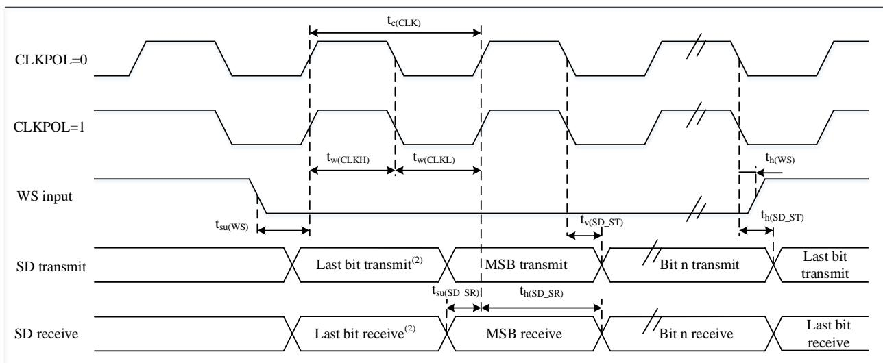
1. The measuring point is set at the CMOS level: 0. 3V<sub>DD</sub> and 0. 7V<sub>DD</sub>.
