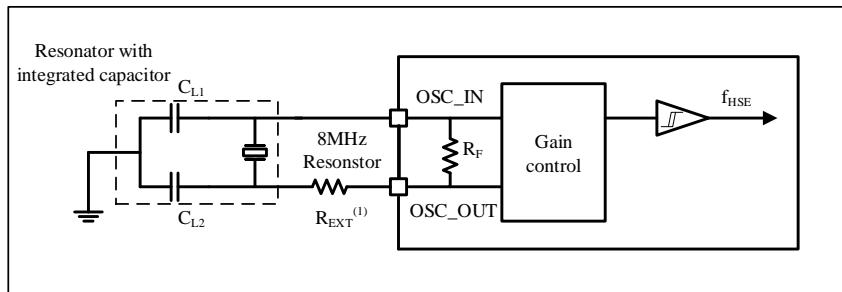
1.  $R_{EXT}$  value is determined by the characteristics of the crystal.
