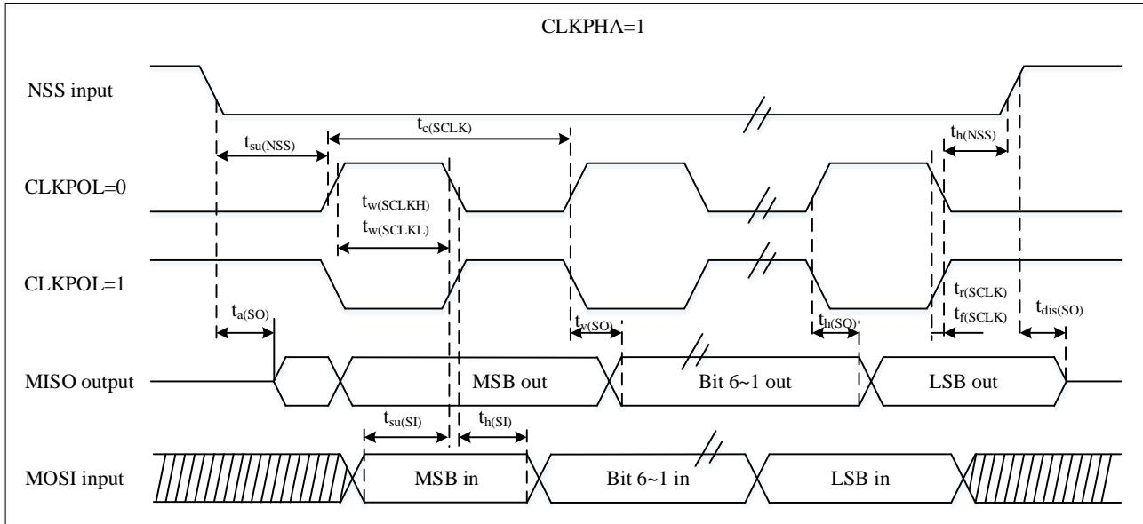
1. The measurement points were set at the CMOS level of 0.3 V<sub>DD</sub> and 0.7 V<sub>DD</sub>.
