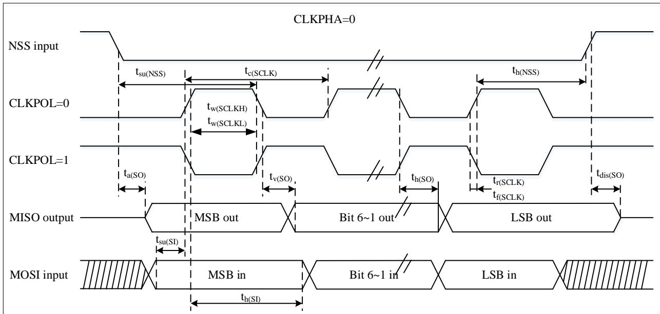
Figure 4-13 SPI sequence diagram - slave mode and CPHA=1<sup>(1)</sup>
