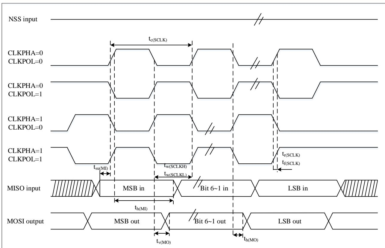
1. The measurement points are set at CMOS level: 0.3 V<sub>DD</sub> and 0.7 V<sub>DD</sub>.
