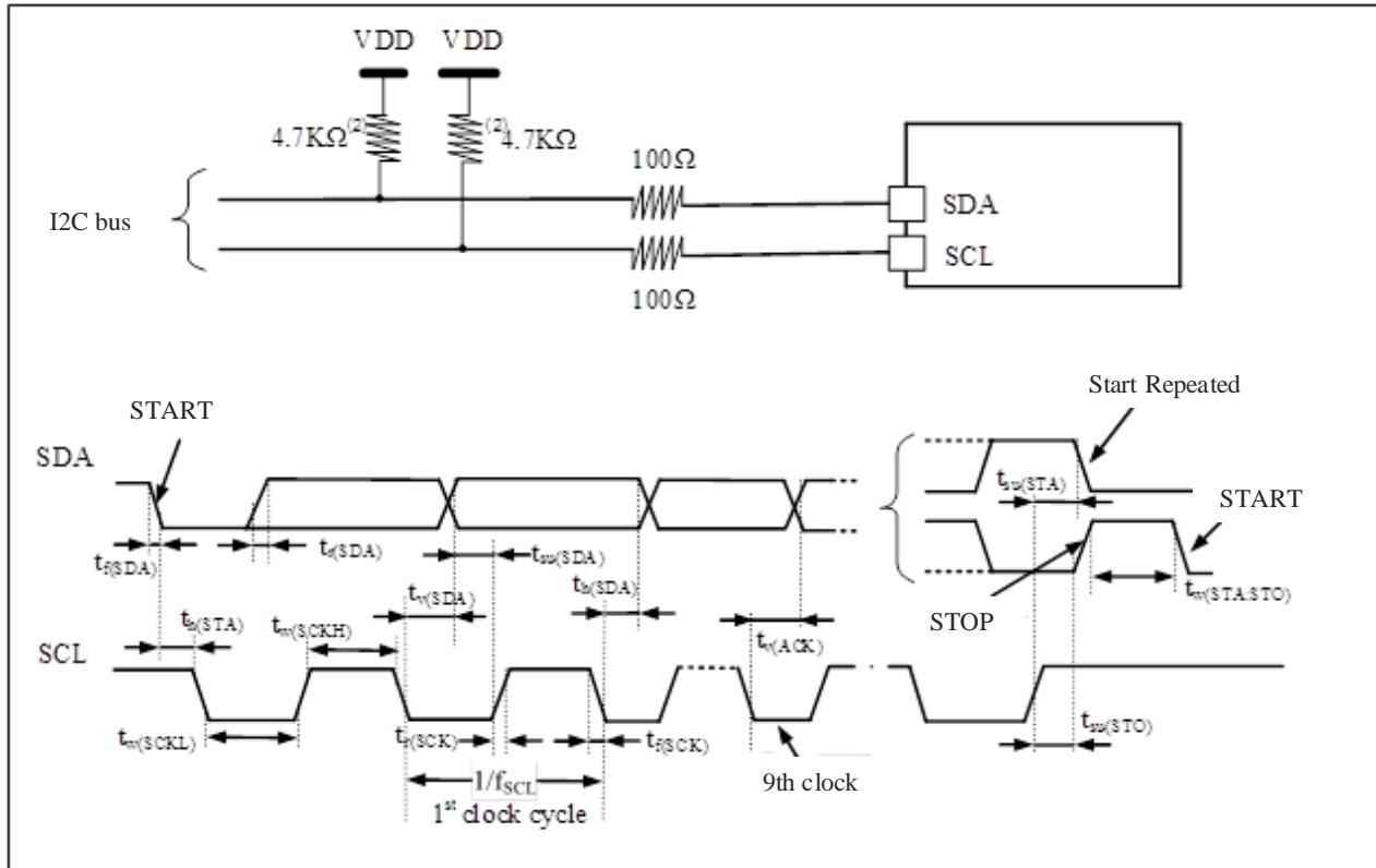
1. The measuring point is set at the CMOS level: 0.3V<sub>DD</sub> and 0.7V<sub>DD</sub>.
