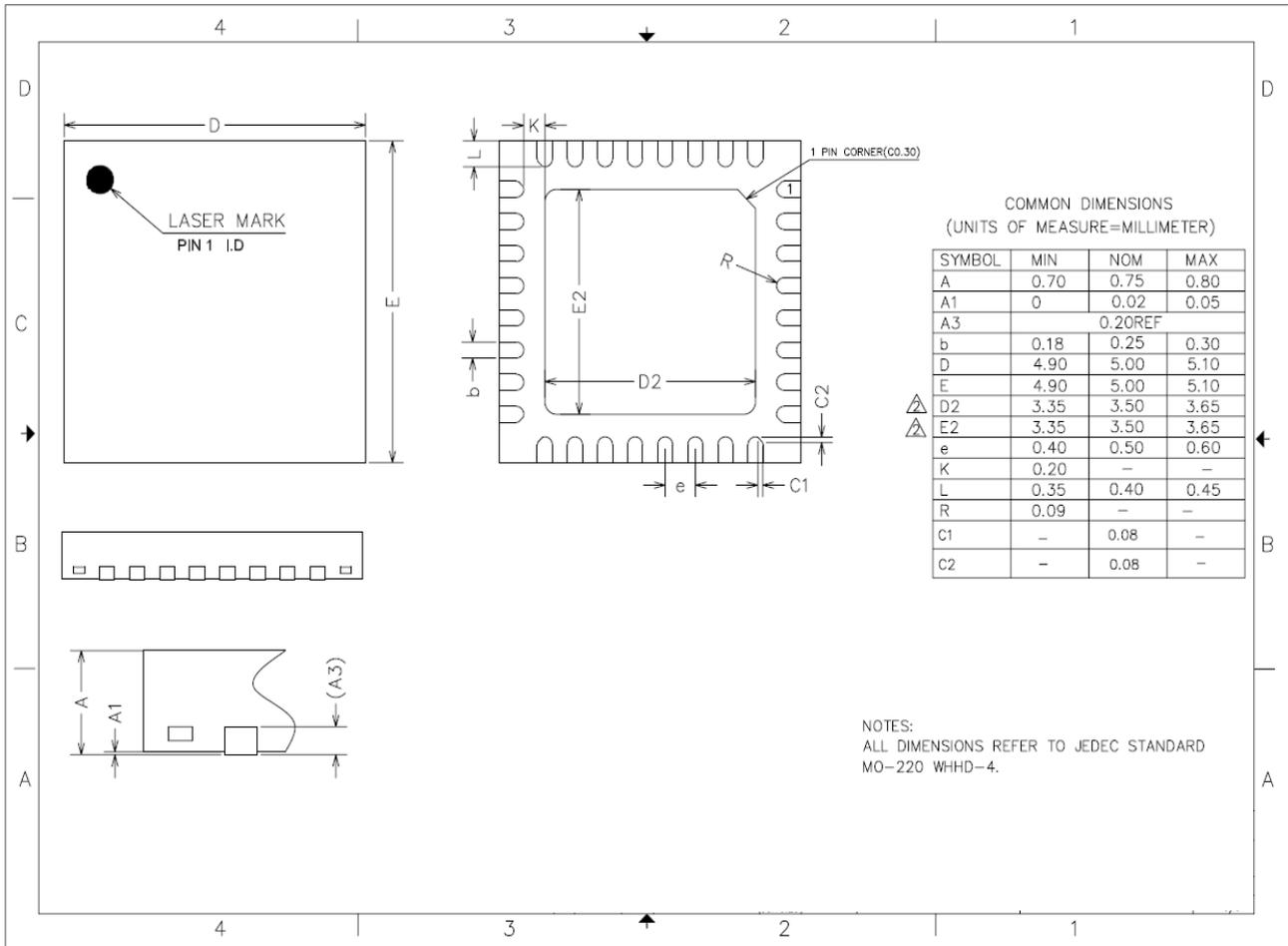
图 5-8 QFP32(5mm x 5mm)封装焊盘建议<sup>(1)</sup>
