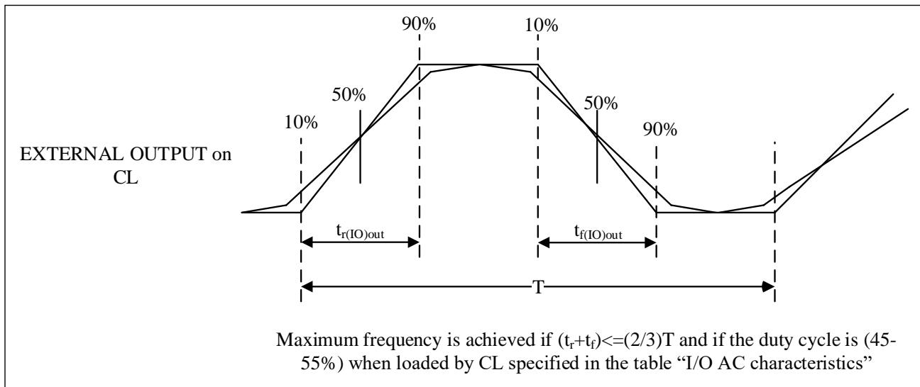
Figure 4-10 Transmission delay
