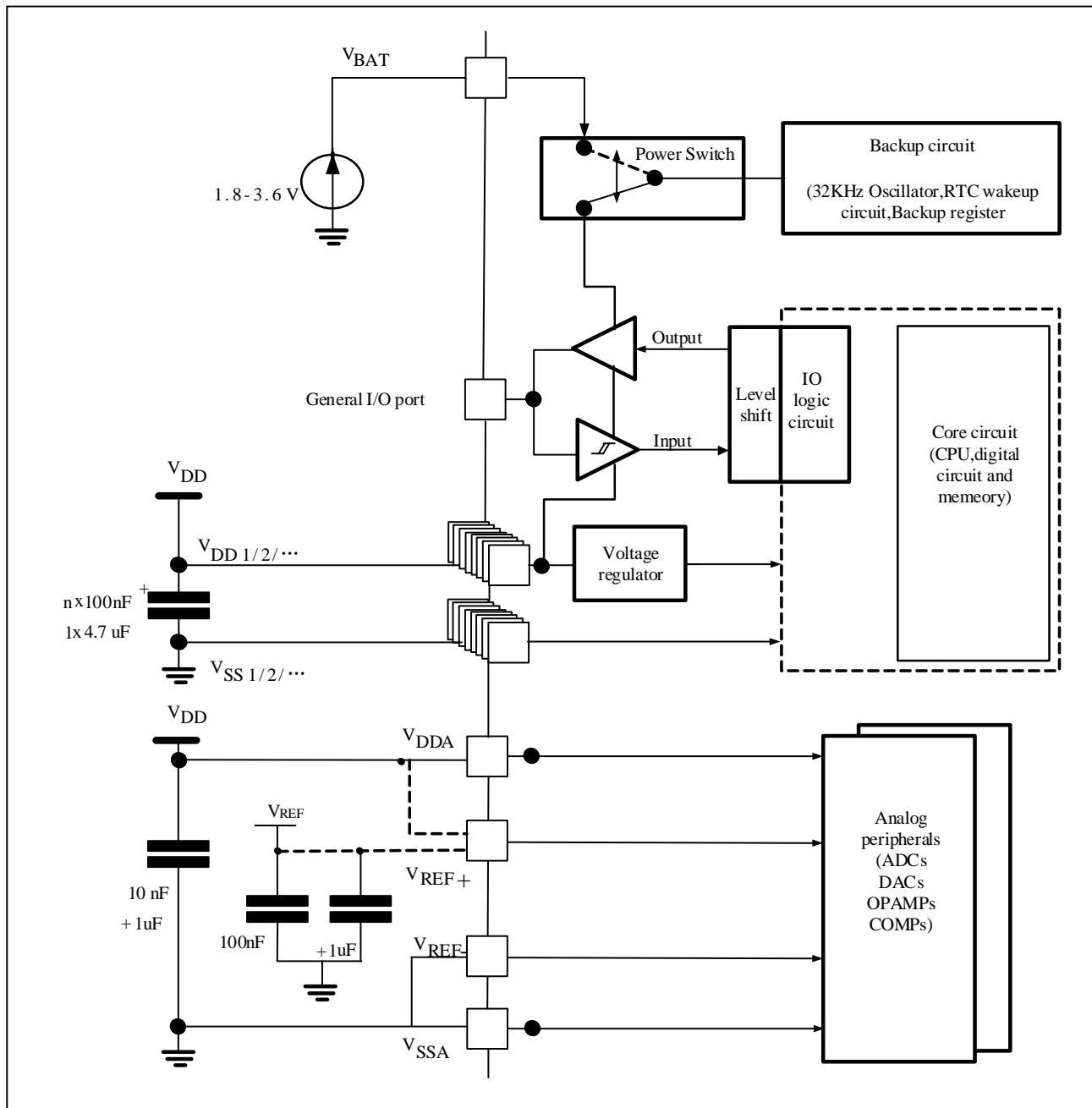
Note: The  $4.7\mu F$  capacitor in the above figure must be connected to  $V_{DD3}$ .
