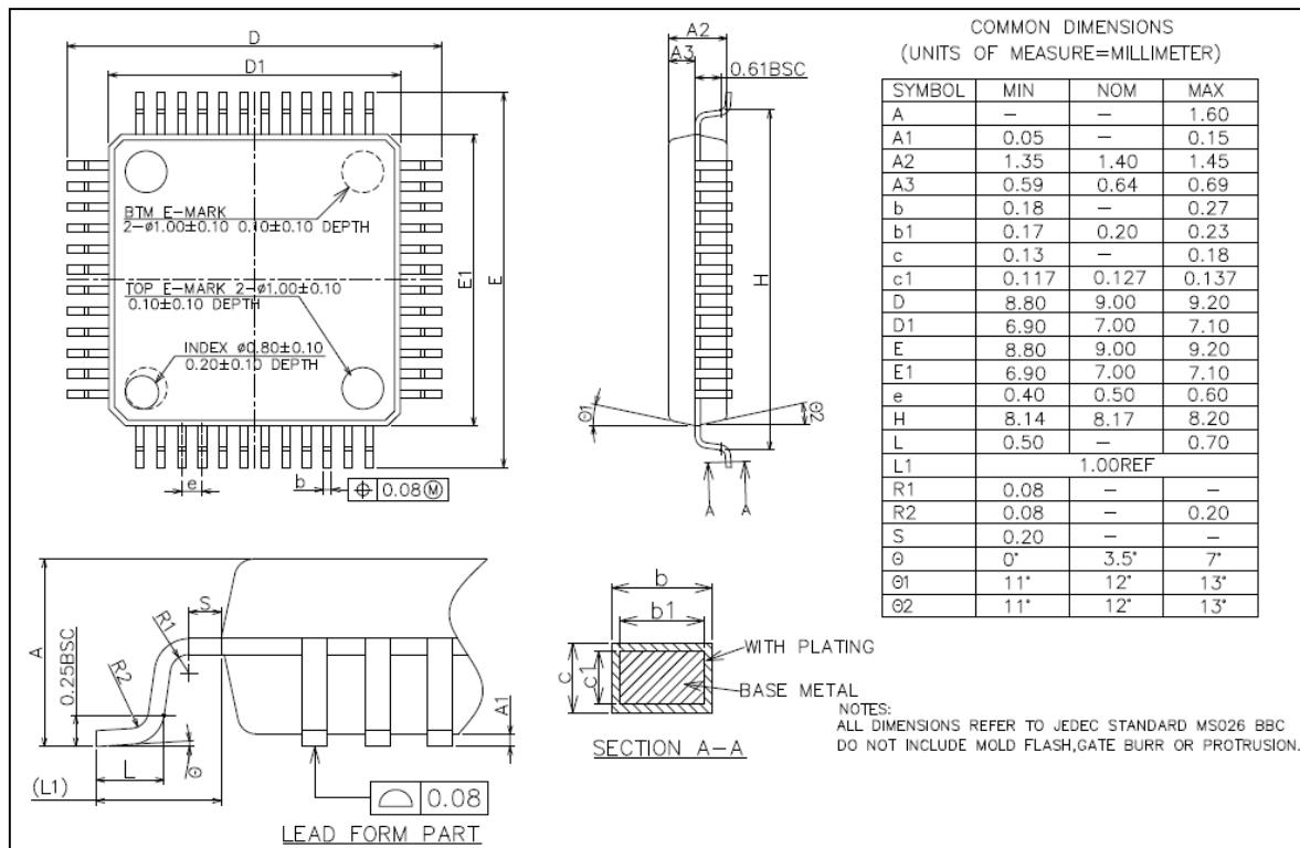
Figure 5-2 LQFP48 recommended footprint<sup>(1)</sup>
