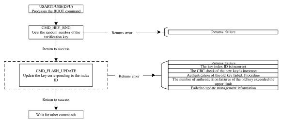
Figure 3.3 command control flowchart for updating a key
