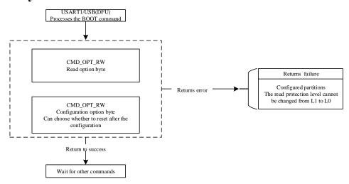
Figure 3.5 flowchart of option byte read/write command control
