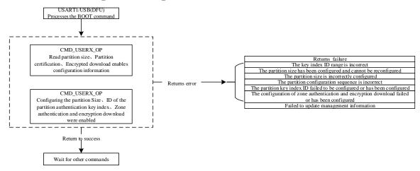
Figure 3.4 Flow chart of commands for Partition Operations
