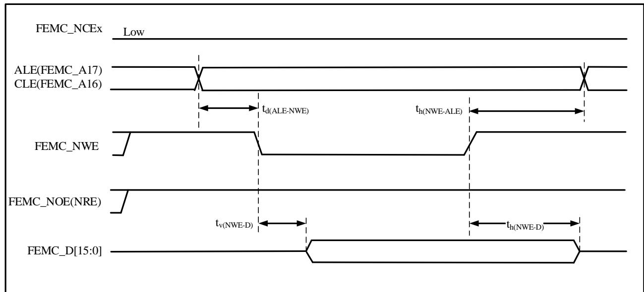
**Figure 4-31 NAND Controller Waveforms For Common Memory Read Access**
