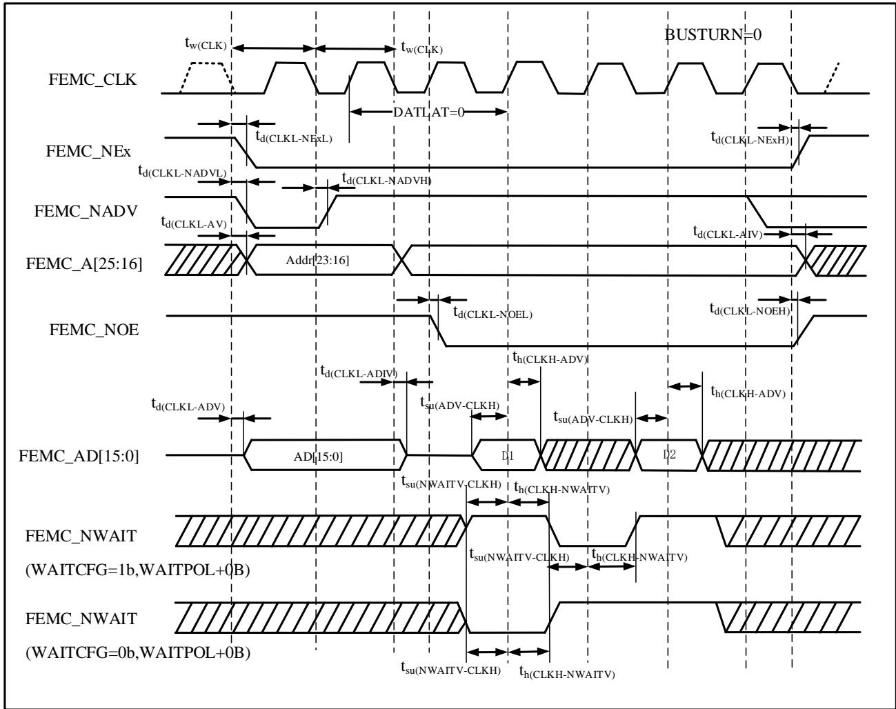
Table 4-55 Synchronous Multiplexed NOR/PSRAM Write Timings<sup>(1)(2)</sup>
