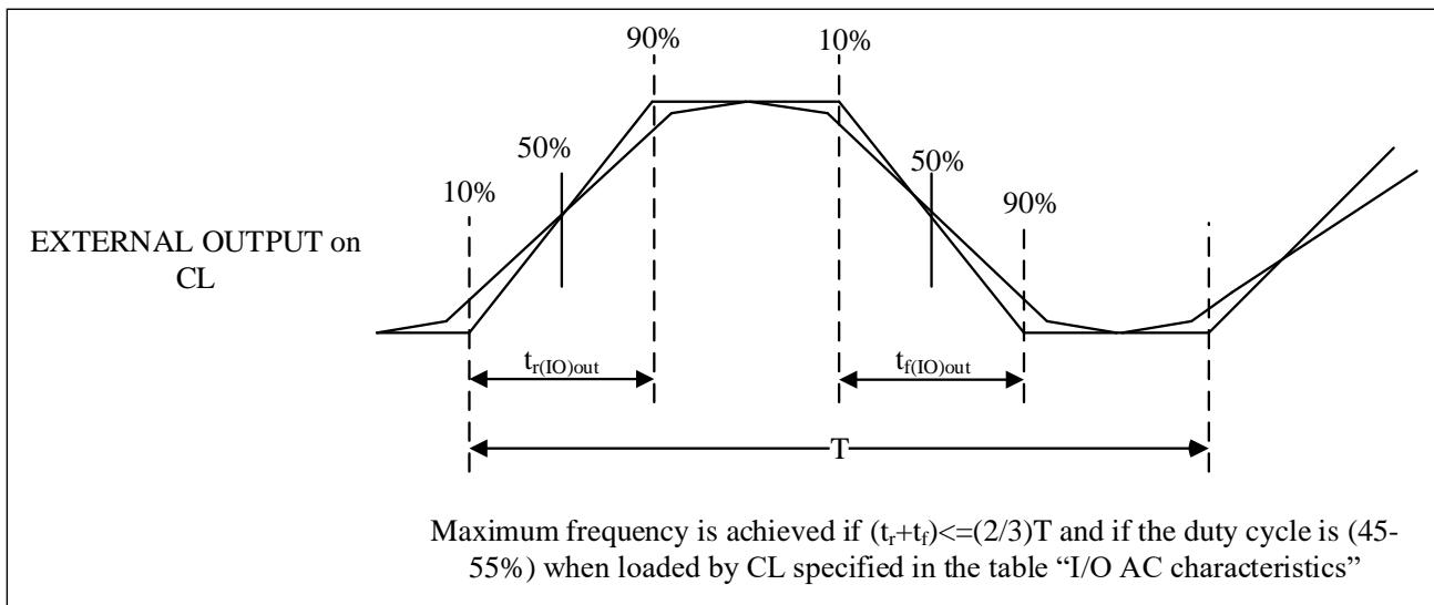
**Figure 4-10 Transmission Delay**
