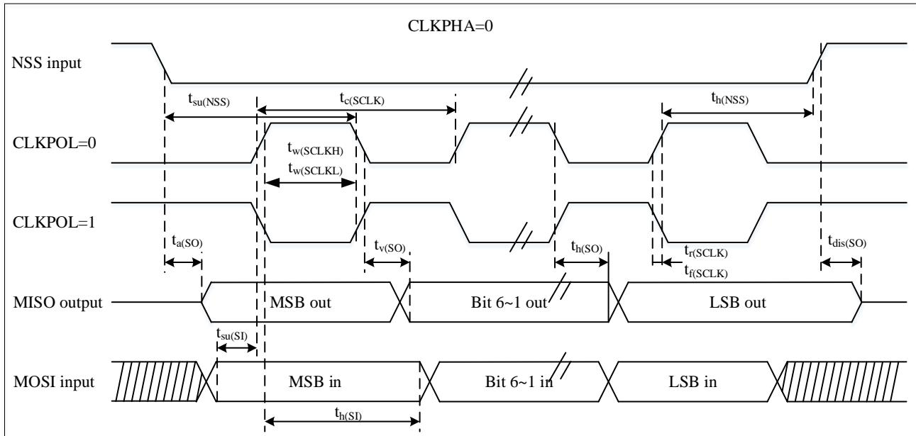
**Figure 4-14 SPI Timing Diagram-Slave Mode And CPHA=1<sup>(1)</sup>**
