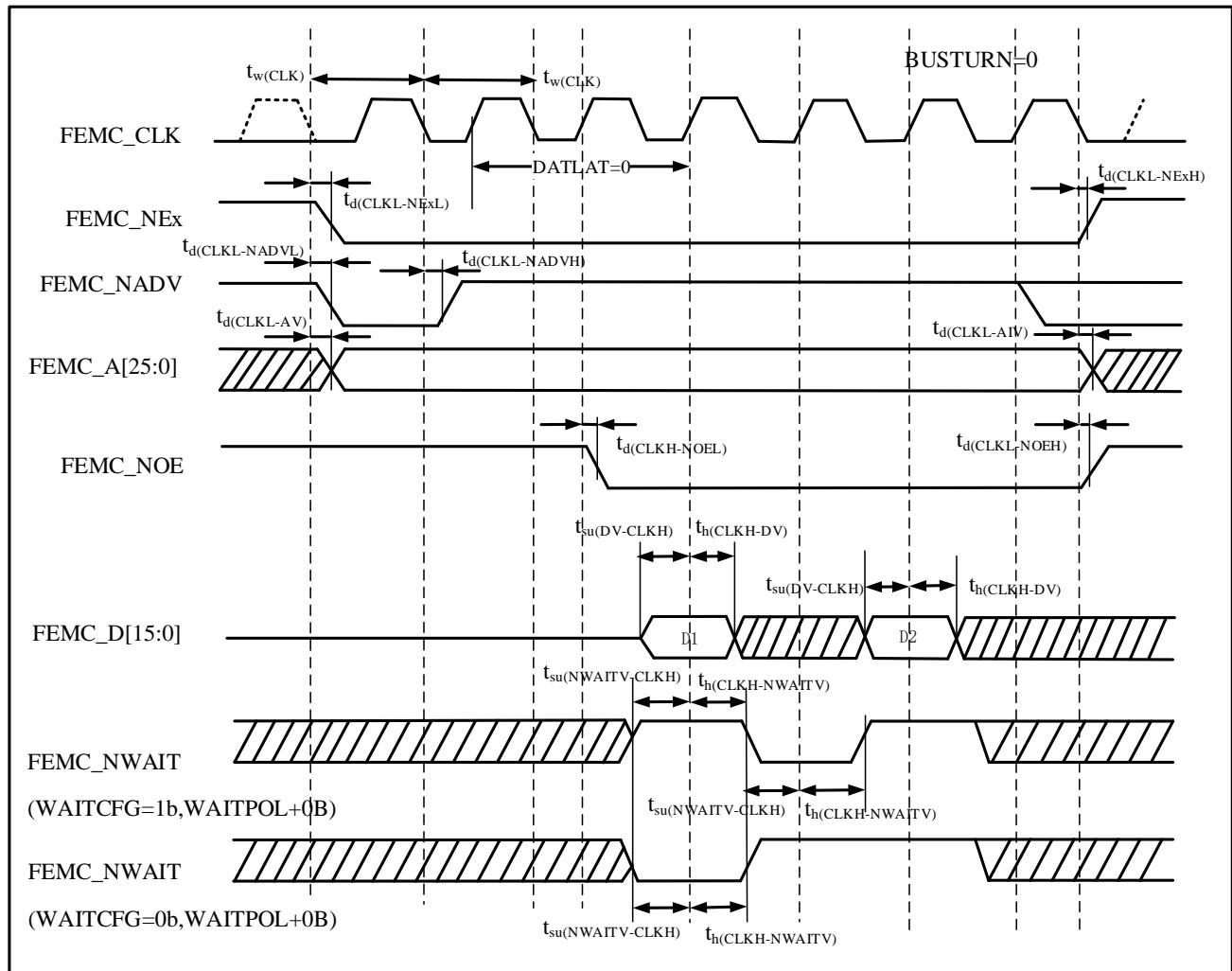
**Table 4-53 Synchronous Non-Multiplexed PSRAM/NOR Read Timings<sup>(1)(2)</sup>**
