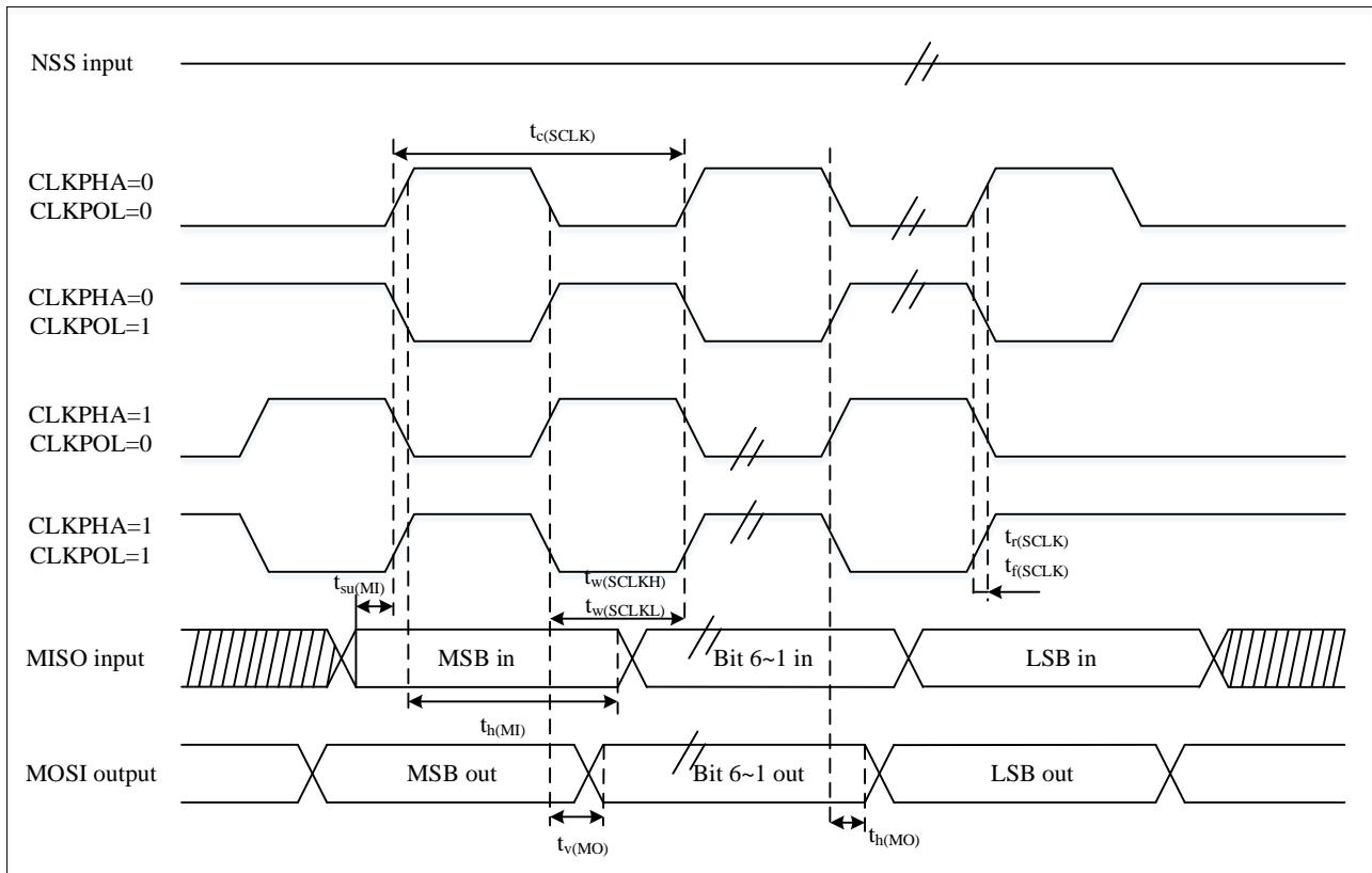
Note: (1) The measuring point is set at the CMOS level: 0.3V and 0.7V<sub>DD</sub>.
