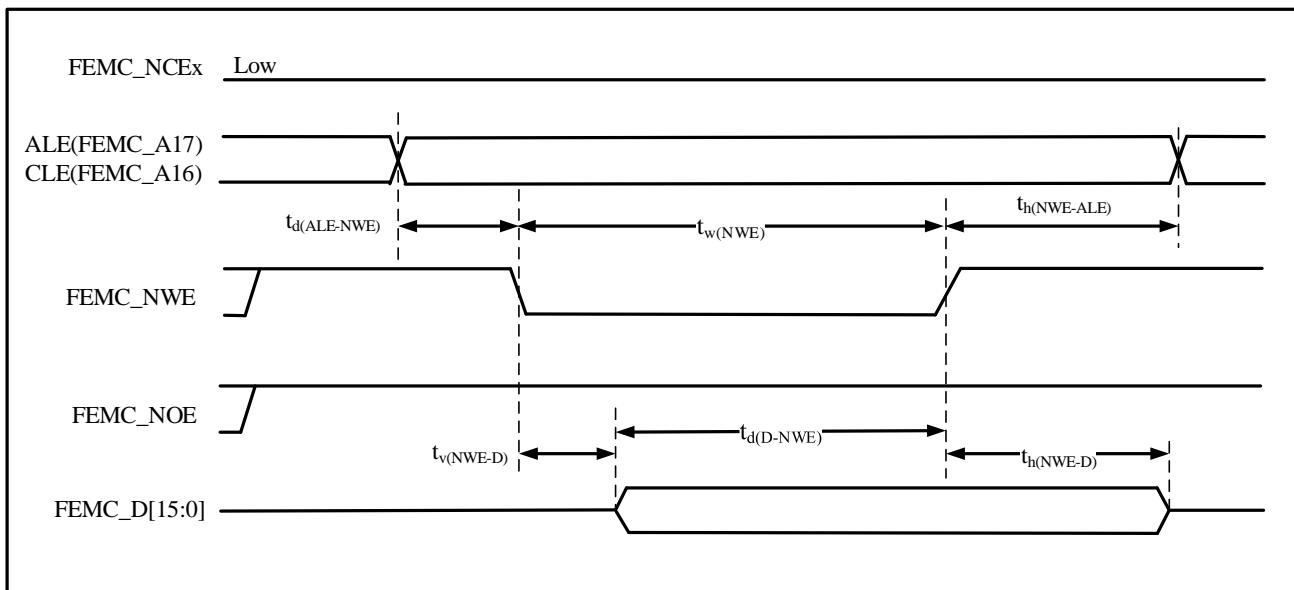
**Table 4-57 Timing Characteristics of NAND Flash Read/Write Cycles<sup>(1)</sup>**
