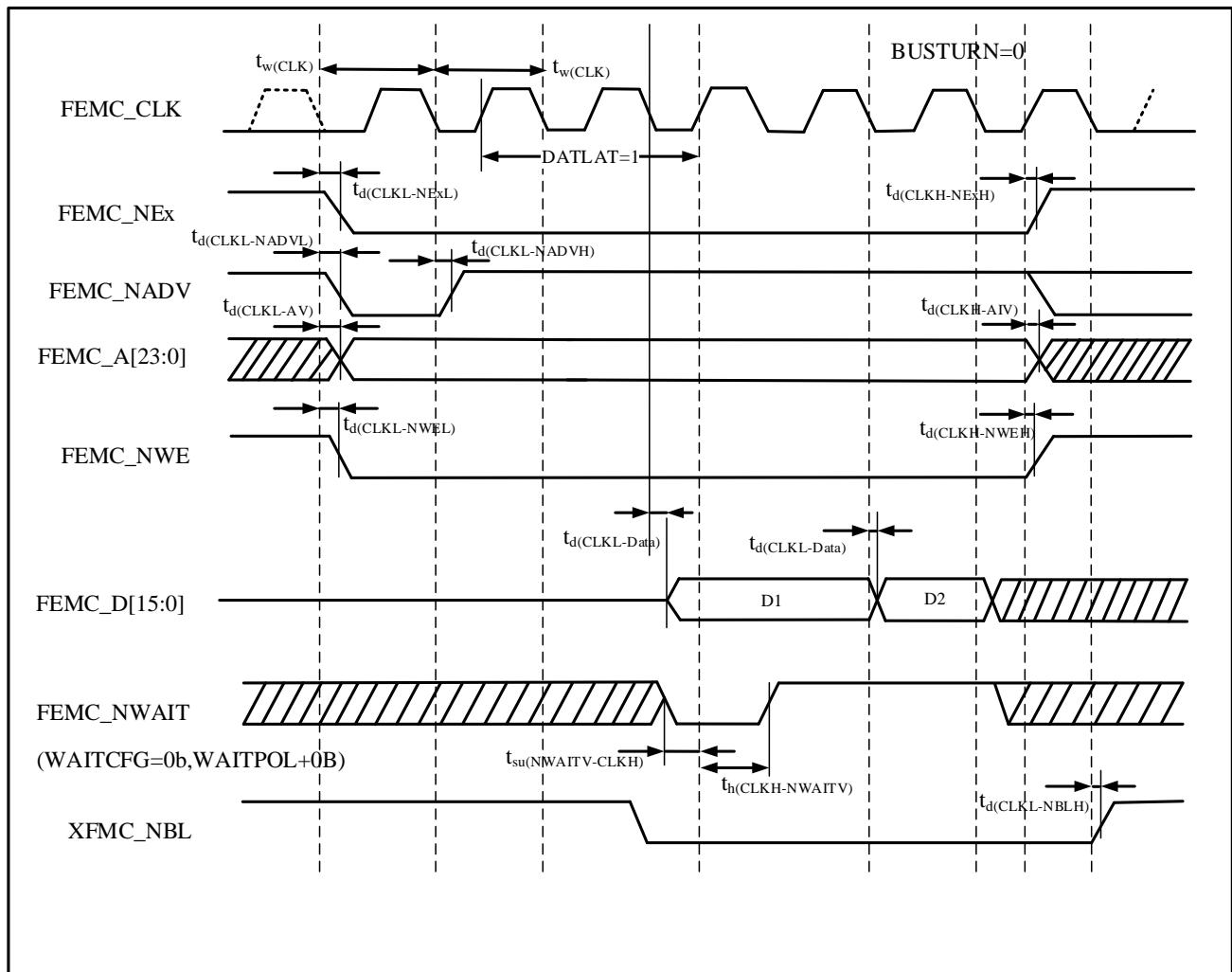
Table 4-54 Synchronous Non-Multiplexed PSRAM Write Timings<sup>(1)(2)</sup>
