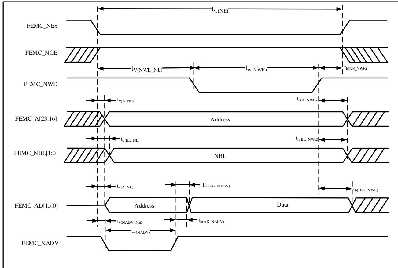
Table 4-52 Asynchronous Multiplexed PSRAM/NOR Write Timings(1)(2)
