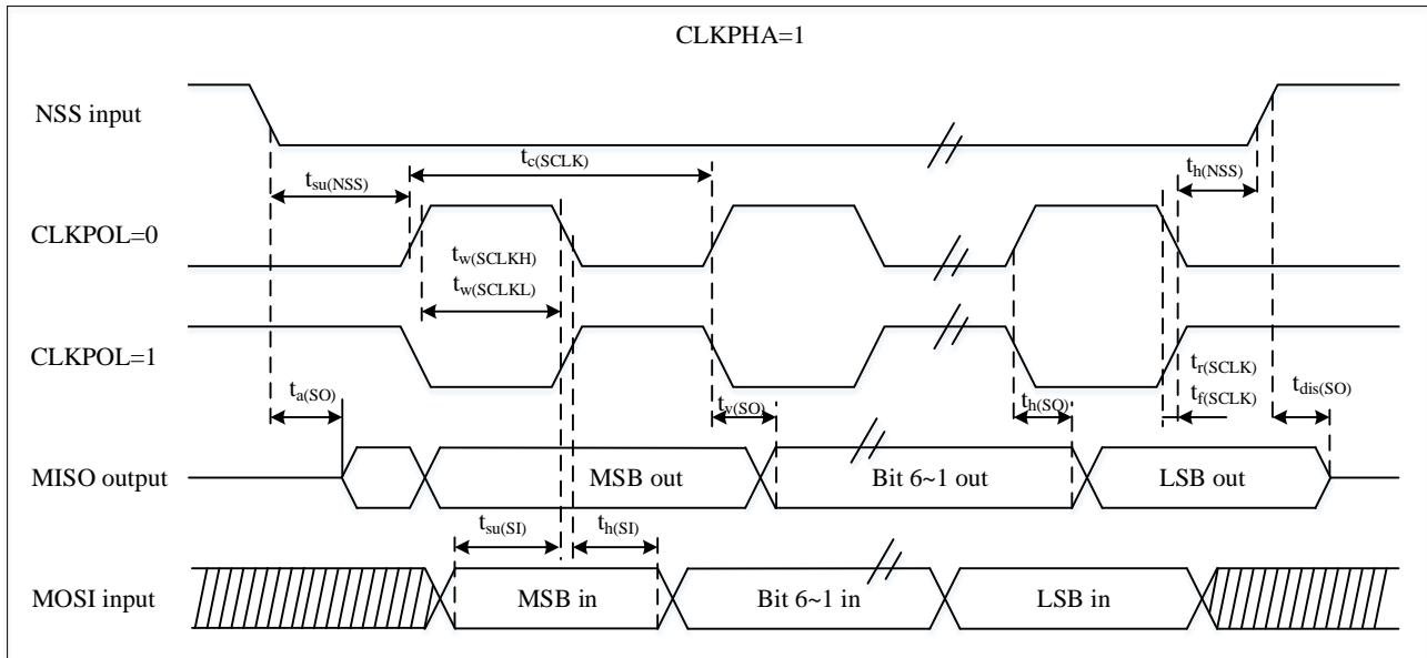
Note: (1)The measuring point is set at the CMOS level: 0.3V<sub>DD</sub> and 0.7V<sub>DD</sub>.
