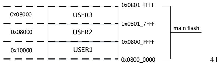
Figure 4-1 Flash main storage area partition relationship
