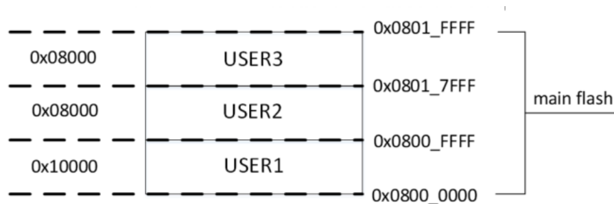
Figure 4-1 Flash main storage area partition relationship
