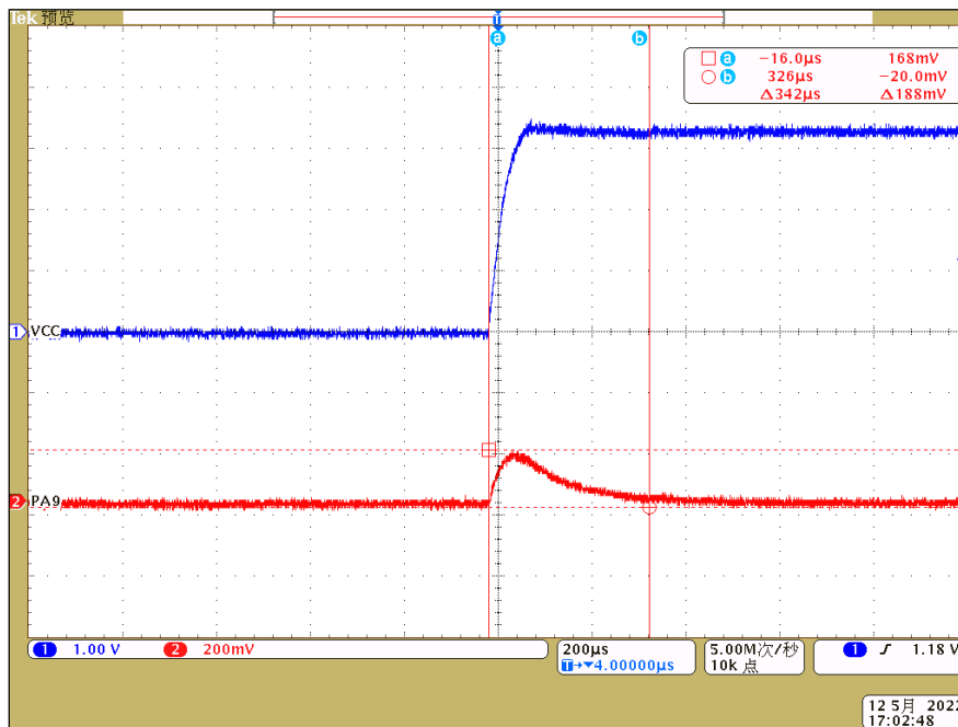
Figure 1-5 IO (PA9) waveform during power-on
