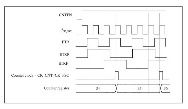
Figure 9-15 Control circuit in external clock mode 2
