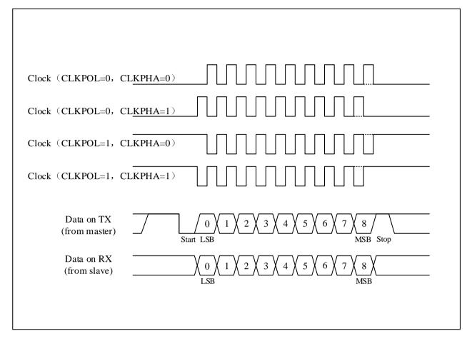
Figure 17-14 RX data sampling / holding time
