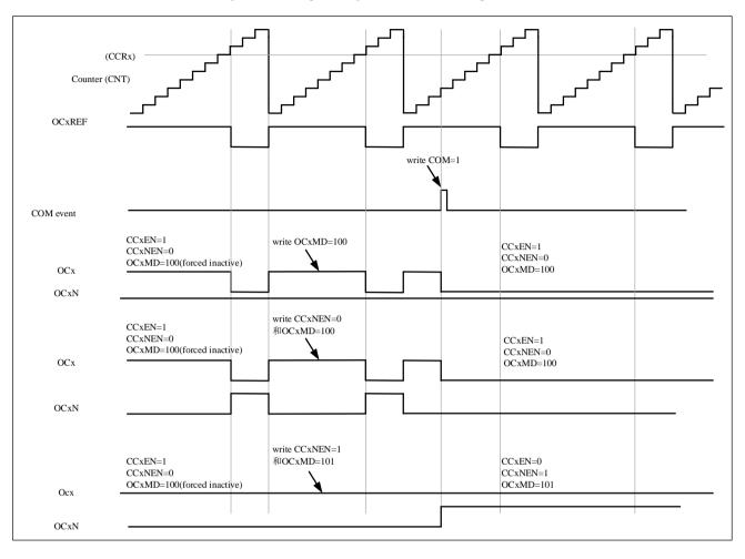
Figure 9-32 6-step PWM generation, COM example (OSSR=1)
