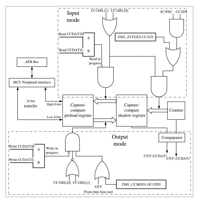
Figure 10-12 Capture/compare channel 1 main circuit
