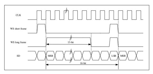
Figure 19-23 PCM standard waveform (16 bits)
