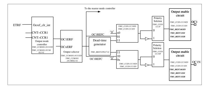
Figure 9-19 Output part of channels (x=4)
