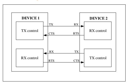
Figure 17-20 hardware flow control between two USART
