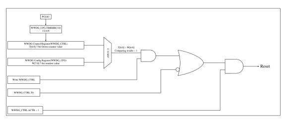
Figure 13-1 Watchdog block diagram
