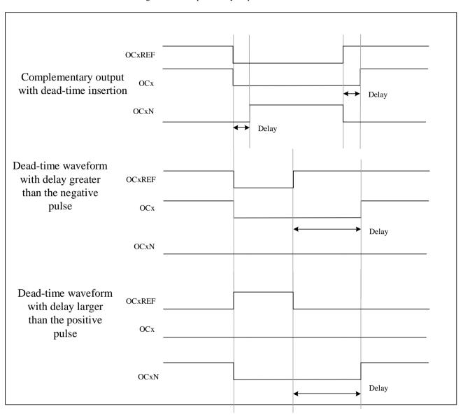
Figure 9-26 Complementary output with dead-time insertion
