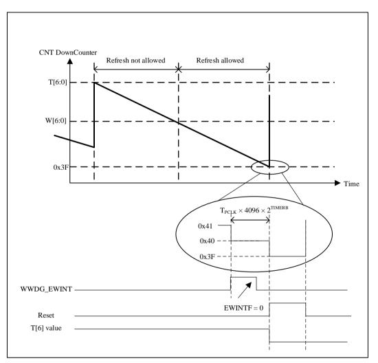
Figure 13-2 Refresh window and interrupt timing of WWDG
