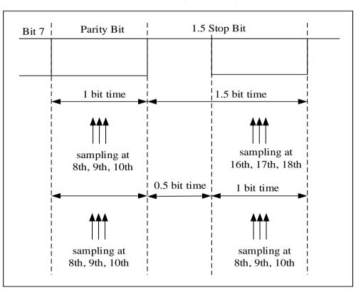
Figure 17-16 Use 1.5 stop bits to detect parity errors
