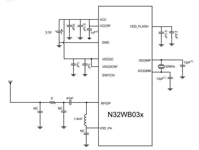
(b) VDCDC/VDCDCRF provided with external power supply
