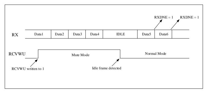
Figure 17-8 Mute mode using idle line detection
