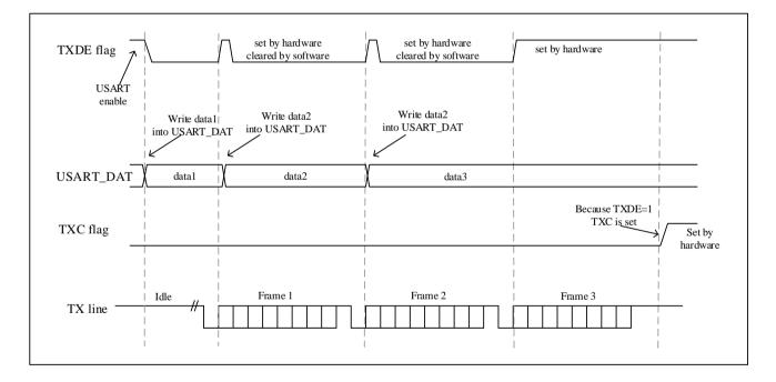
Figure 17-4 TXC/TXDE changes during transmission
