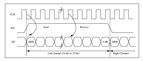
Figure 19-19-17 The MSB is aligned with 16-bit or 32-bit full precision, CLKPOL = 0.
