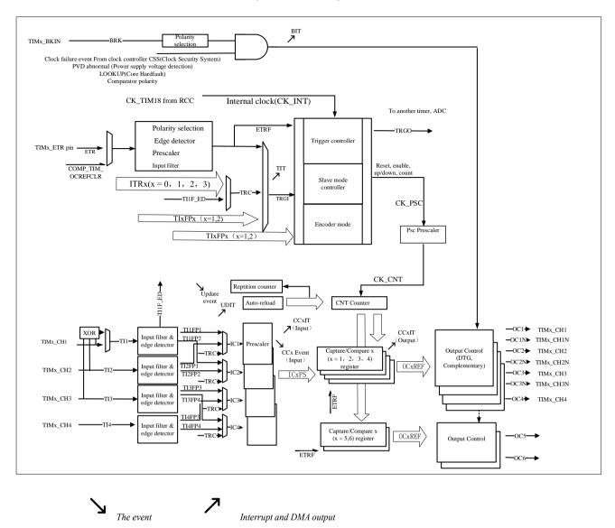
The capture channel 1 input can come from IOM or comparator output
