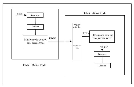
Figure 10-20 Block diagram of timer interconnection
