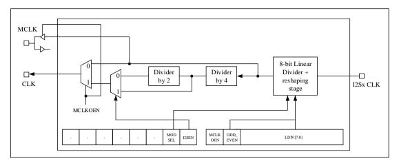
Note: The clock source of  $I^2Sx$  CLK is HSI, HSE or PLL system clock that drives AHB clock.
