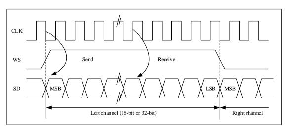
Figure 19-19-20 LSB alignment 16-bit or 32-bit full precision, CLKPOL = 0
