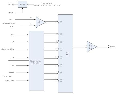
Figure 15-1 Architecture diagram of voice control and ADC
