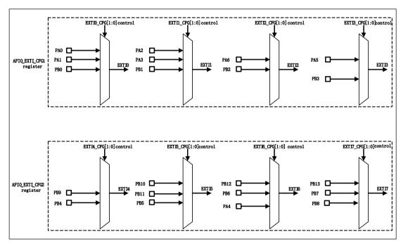
To configure external interrupts/events on the GPIO line using AFIO\_EXTI\_CFG1~2, the AFIO clock must be enabled first. Universal I/O ports are connected to 8 external interrupt/event lines as shown above. The connection mode of the other 6 EXTI lines is as follows:
