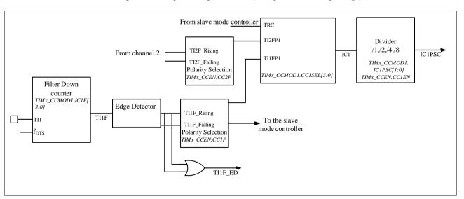
Figure 10-11 Capture/compare channel (example: channel 1 input stage)
