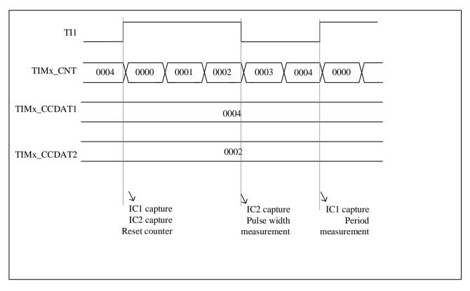
Because of only filter timer input 1 (TI1FP1) and filter timer input 2 (TI2FP2) are connected to the slave mode controller, the PWM input mode can only be used with the TIMx\_CH1/TIMx\_CH2 signals.
