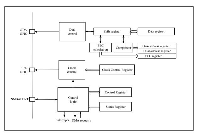
Note: in SMBus mode, SMBALERT is an optional signal. If SMBus is disabled, the signal cannot be used.
