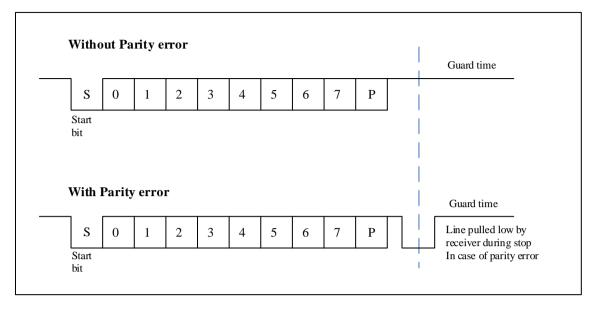
When connecting with a smart card, the TX pin needs to be set to open-drain mode, and an external pull-up resistor is connected. This pin will drive the same bidirectional connection with the smart card. During the data byte, it is released (weak pull-up) during the transmission of the stop bit, so the receiver can pull the data line low in case of parity error. If TXEN is not enabled, TX will be pulled high during the stop bit.
