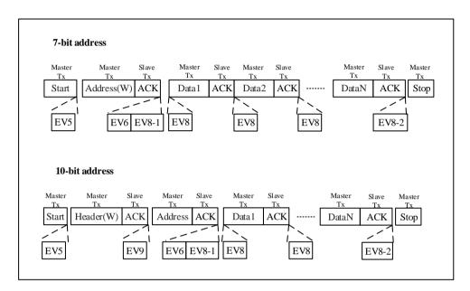
Figure 16-2 Master transmitter transfer sequence diagram
