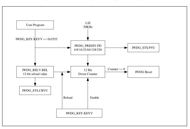
Figure 12-1 Functional block diagram of the independent watchdog module
