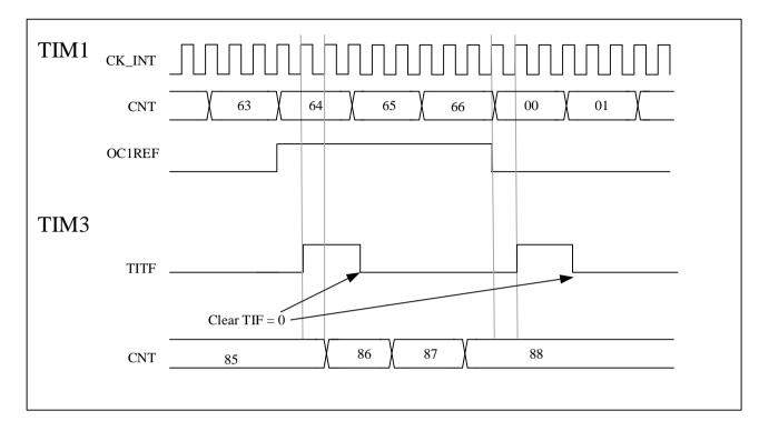
In the next example, Gated TIM3 with enable signal of TIM1, Setting TIM1.CTRL1.CNTEN = '0' to stop TIM1. TIM3 counts on the divided internal clock only when TIM1 is enable. The clock of both counters are based on CK\_INT via a prescaler divide by 3 is performed ( $f_{CK_CNT} = f_{CK_INT}/3$ ).
