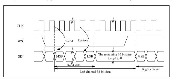
Figure 19-19-16 I<sup>2</sup>S Philips protocol standard waveform (16-bit extended to 32-bit packet frame, CLKPOL = 0)
