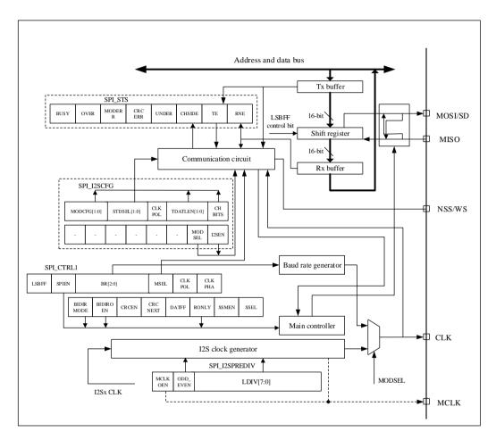
The I2S interface uses the same pins, flags and interrupts as the SPI interface. Setting the MODSEL = 1 selects the I2S audio interface.
