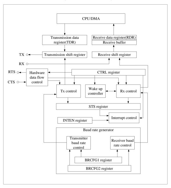
Figure 18-18-1 LPUART block diagram
