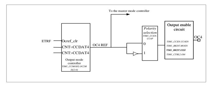
Reads and writes always access preloaded registers when capturing/comparing. The two specific working processes are as follows:
