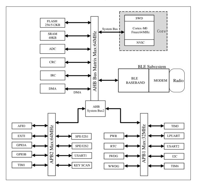
Figure 2-1 Architecture Diagram of System Bus
