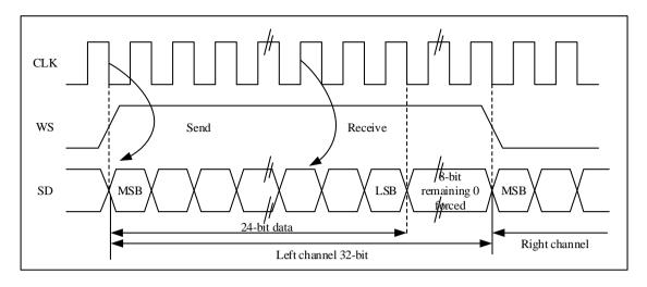
Figure 19-19 MSB-aligned 16-bit data is extended to 32-bit packet frame, CLKPOL = 0
