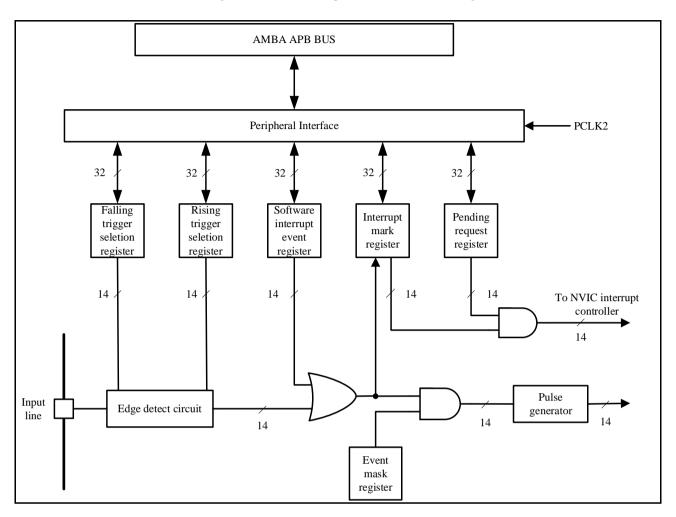
Figure 6-1 Extenal interrupt/event controller block diagram
