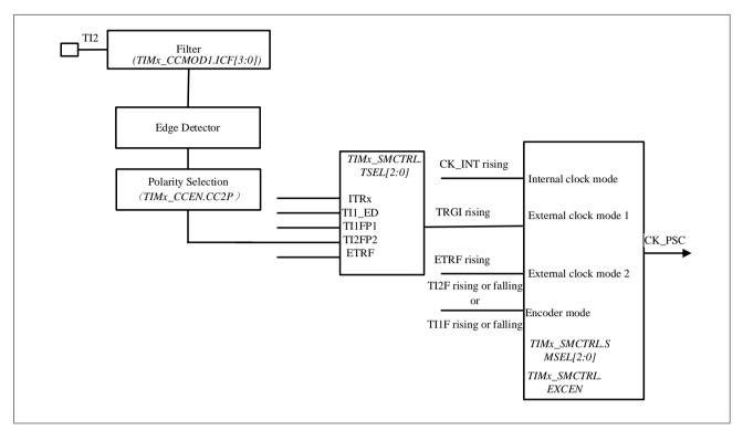
This mode is selected by configuring TIMx\_SMCTRL.SMSEL=111. The counter can be configured to count on the rising or falling edge of the clock at the selected input.
