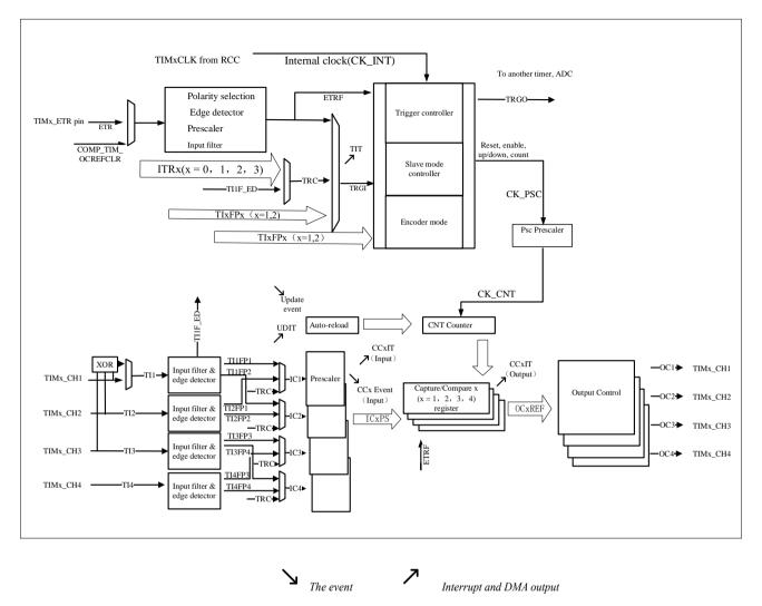
The capture channel 1 input can come from IOM or comparator output
