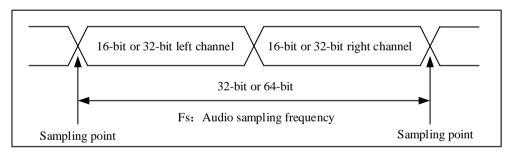
Audio can be sampled at 96kHz, 48kHz, 44.1kHz, 32kHz, 22.05kHz, 16kHz, 11.025kHz, or 8kHz (or any value within this range). Set the linear divider by referring to the following formula:
