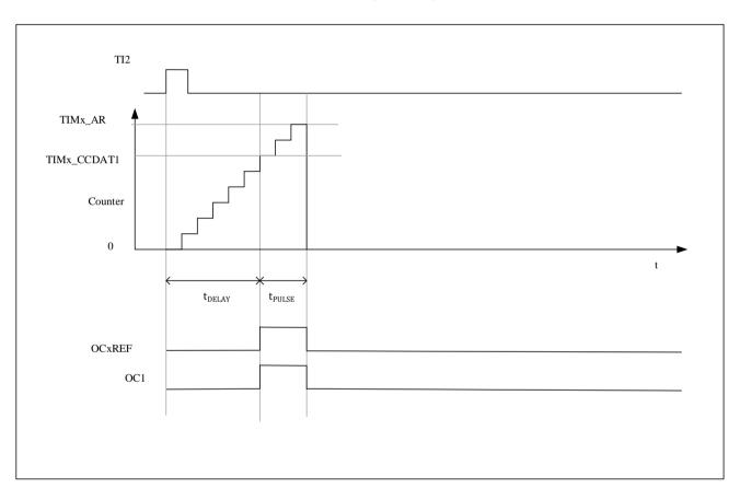
Figure 9-24 Example of One-pulse mode
