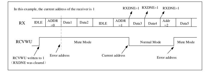
Figure 17-4 Mute mode detected using address mark
