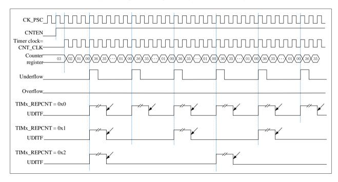
Figure 9-8 Repeat count sequence diagram in down-counting mode
