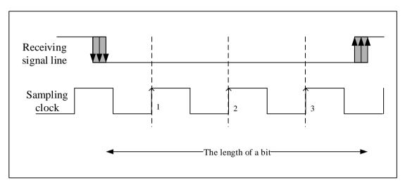
Figure 18-18-4 Data sampling for noise detection
