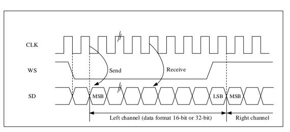
Figure 19-19-14 I<sup>2</sup>S Philips protocol waveform (16/32-bit full precision, CLKPOL = 0)
