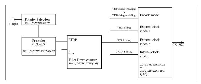
For example, use the following configuration steps to make the up counter count every 2 rising edges on ETR.
