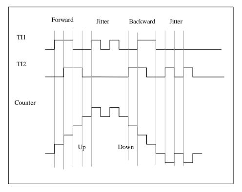
The following figure shows the example of counter behavior when IC1FP1 polarity is inverted (CC1P= '1', other configurations are the same as above)
