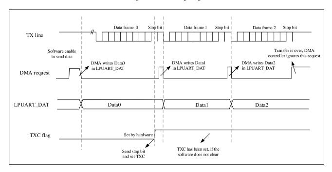
Figure 18-18-5 Sending using DMA
