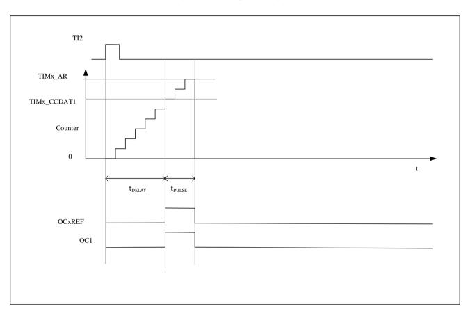
Figure 10-18 Example of One-pulse mode
