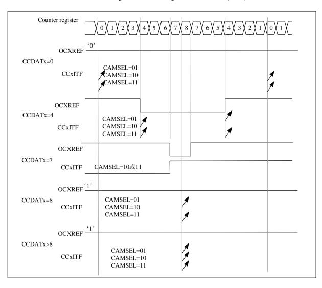
Figure 10-16 Center-aligned PWM waveform (AR=8)
