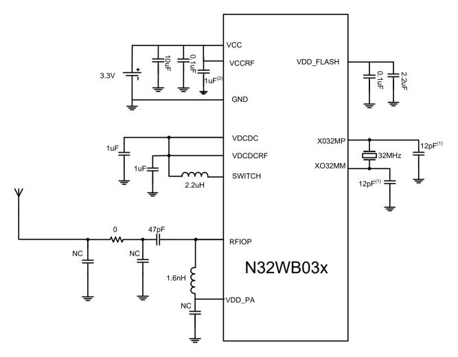
(a) VDCDC/VDCDCRF provided with internal DCDC power supply
