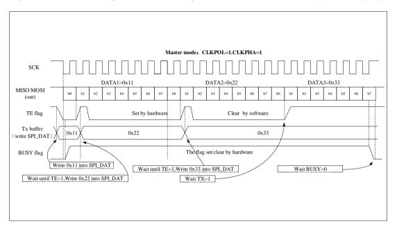
Figure 19-19-6 Schematic diagram of TE/BUSY change when the host transmits continuously in one-way only mode
