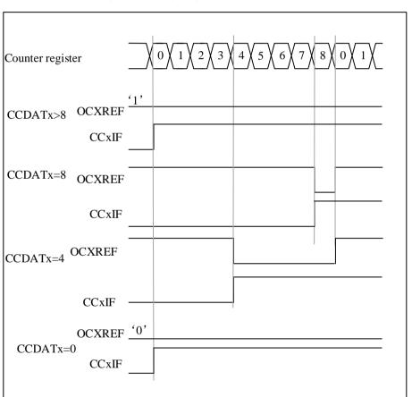
Figure 10-17 Edge-aligned PWM waveform (APR=8)
