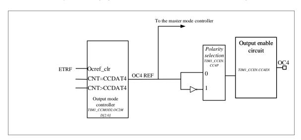
Figure 10-13 Output part of channels (x = 1,2,3,4; take channel 4 as an example)
