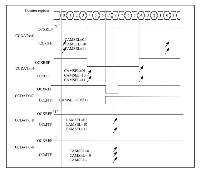
Figure 9-22 Center-aligned PWM waveform (AR=8)
